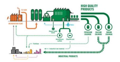
In the first step, fly ash is washed with water. This removes washed ash (residual sand), leachate containing salt and a small amount of metals. The metals are then removed with sulphides from the leachate, where the liquid with the dissolved salts continues to the second stage: salt separation.
